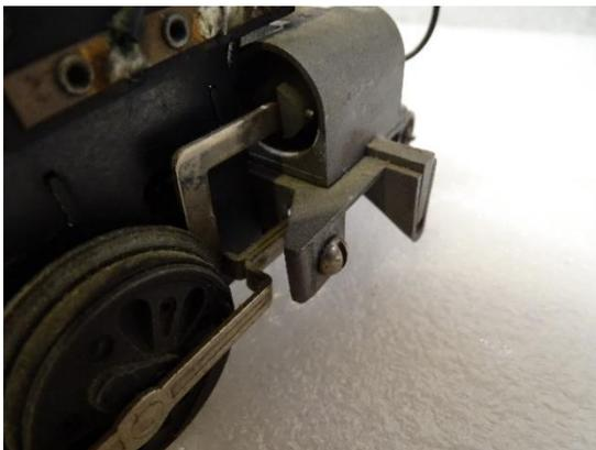
The piston for the steam chest may warp or melt. RG Part No. 305 Smoke Unit Nylon Piston is available to replace a damaged part.
