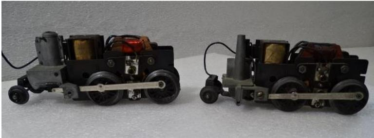
A Marx 1666 steam chest smoker engine (right) compared to a standard 666/1666 smoker engine (left). The standard smoker engine has a trim piece (RG Part No. 212 666/1666 Smoke Unit Top Insert) at the top to extend the stack up through the engine shell's smokestack. The steam chest smoker's stack has a tapered smokestack and does not accommodate an insert trim piece.
