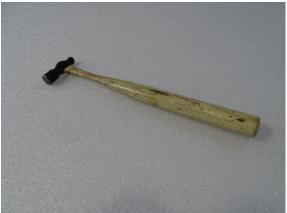
A small ball peen hammer provides enough force when lightly tapped to gently mushroom the post over the side rod.
