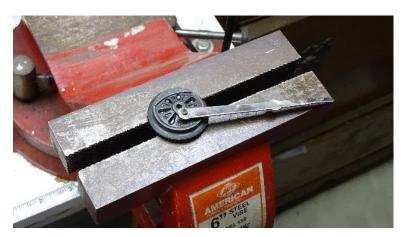
Place the driver wheel in a vise, with the post over the jaw before beginning to re-install a side rod.
