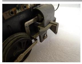
The piston for the steam chest may warp or melt. RG Part No. 305 Smoke Unit Nylon Piston is available to replace a damaged part.
