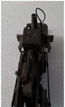
**Note:** Marx had a common smoke unit that came in most 666/1666 engines. The common smoke unit uses the RG Part No. 310 side rod with pin, which is not compatible with the steam chest motors.
